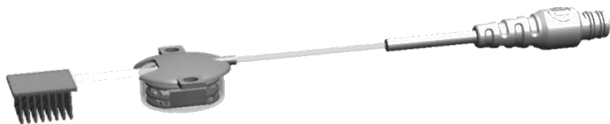
FIGURE 4: FINAL SATELLITE ASSEMBLY FITS IN A 14-MM DIAM HERMETIC ENCLOSURE DESIGNED TO SIT WITHIN A STANDARD CRANIAL BURR-HOLE. THE SATELLITE CAN BE ATTACHED TO ANY VARIETY OF ELECTRODE TYPES.
